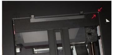
Kodak Disc Film Holder: Note: Disc holders sold after 10/8/19 do not require removing the center hub! Make sure frame numbers are facing down towards the scanner.
